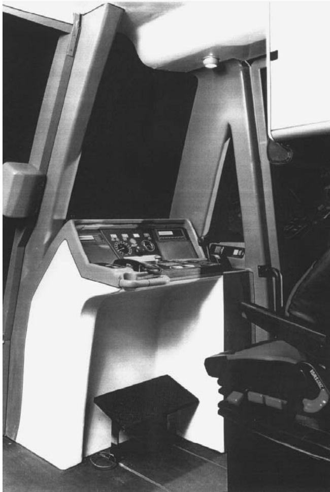
FIGURE 28.25 Full size mock-up of the Express Train cab constructed for user trials in Hong Kong.
