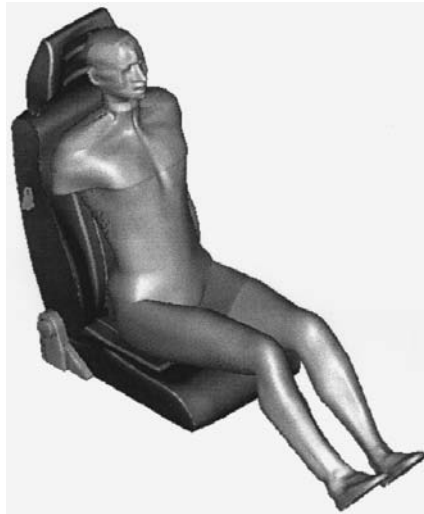
FIGURE 28.8 SAMMIE model of an individual person recorded by the LASS bodyscanner system.
