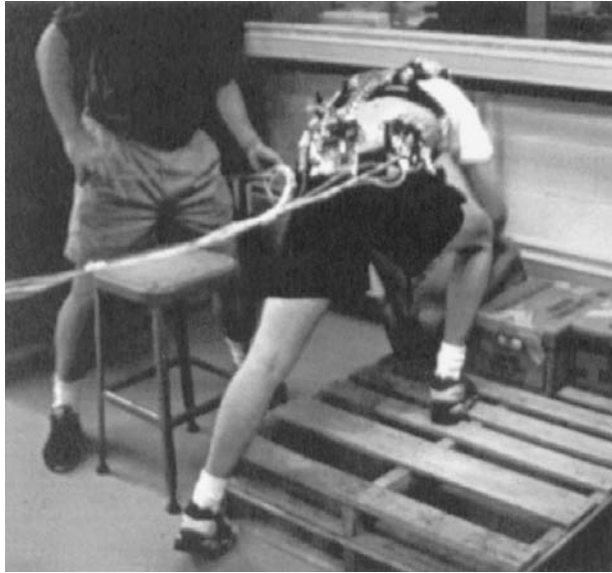
FIGURE 22.6 An order selector performing a stock picking task and wearing the experimental apparatus required to perform an LMM risk analysis and EMG-assisted model analysis.
