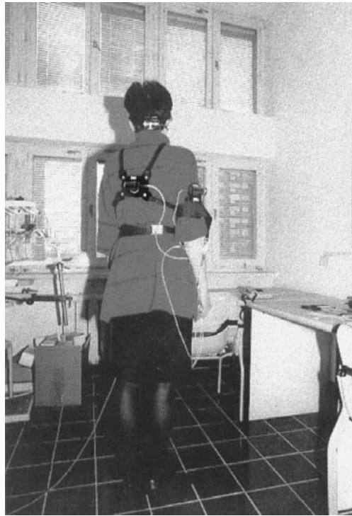
FIGURE 31.17 Pendulum potentiometer sensors placed on the head, back, and arm.
