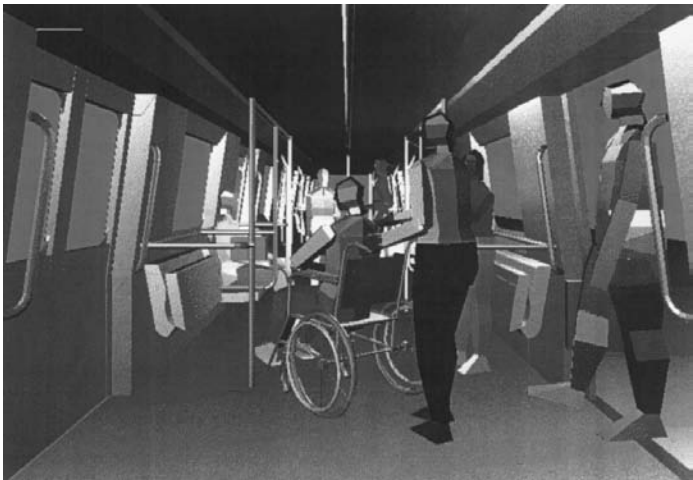
FIGURE 28.5 SAMMIE models used to evaluate accommodation in a railway carriage. (Source: Loughborough University web page.)
