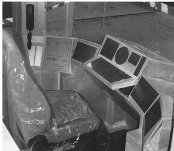
FIGURE 28.20 This mock-up of the Amsterdam Tram was made exactly to the SAMMIE specification and successful trials with Dutch drivers were conducted.
