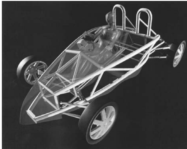
FIGURE 28.18 SAMMIE model ported into Alias for developing the styling and engineering around the defined future occupants. (Photograph courtesy of Dr. C.S. Porter, Coventry University, UK.)
