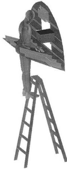
FIGURE 28.1 MDHMS model of an aircraft maintenance operation. (Source: MDHMS web page.)
