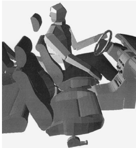
FIGURE 28.9 SAMMIE evaluation of the Fiat Punto before full-size prototypes were available for road trials.
