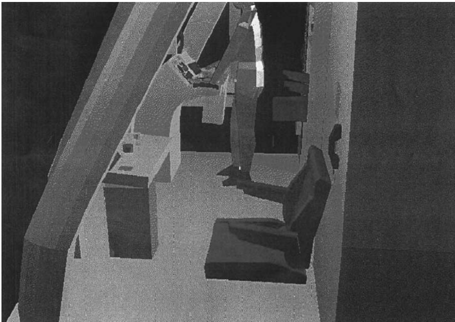
FIGURE 28.24 SAMMIE model of the Express Train cab showing the sit/stand workstation with the seat recessed to improve cross cab access.
